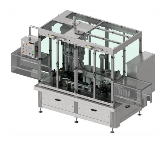
Closing Rotational Module ZIGMAT Z-1422 is part of an automatic aerosol production line and is designed to drop aerosol valves into containers and then clamp them onto the containers. The process is carried out by a valve insertion module and a rotary closing station equipped with 9 actuators.
