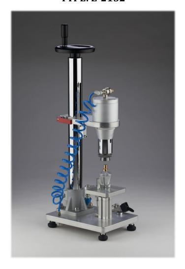
Semi-automatic crimping machine Z-2152 is a device used for a tight and reliable crimp of atomizers on glass bottles which are provided manually. Device is powered and controlled by compressed air only. Reliable embedment of atomizer on glass container is conducted by crown-shaped crimp on atomizer's collar. Proper configuration of head height, working pressure and crimp parameters guarantees the correctness of the whole cycle.
