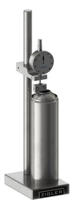
PPCP is a measuring instrument for controlling the parallelism of an aerosol container opening's plane with respect to its base plane. It is intended to be used with the aluminum and steel aerosol cans. According to EN 15010 standard, the parallelism of the aerosol can is considered 1 of 3 critical parameters directly related with the effectiveness of aerosol valve crimp, thus is defining the quality of end aerosol product.
