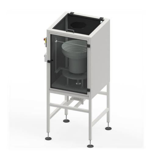
Vibratory Sorter is a machine for feeding appropriately oriented elements (sprayheads, caps, valves) to the inserting/closing machine. The upper part of the sorter comprises a feeding hopper, where, under the influence of controlled vibrations and properly shaped spiral track, elements are oriented and fed to the slideway. The machine is equipped with dedicated control cassettes to control operation of Vibratory Sorter.
