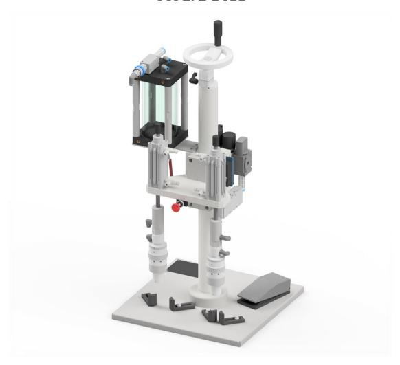
Semi-automatic Vacuum Filling Machine Z-2411 is a device which intended use is to fill glass bottles with liquid product. Bottles are provided manually. The use of vacuum mechanism allows to maintain equal level of liquid in each bottle, regardless of volume differences (even very small - being a result of glass thickness differences). Device is equipped with its own vacuum generator and with drain tank, where excess of liquid is stored during liquid leveling in bottles.
