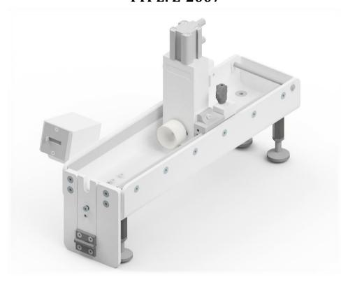
Semi-automatic Tubes Cutter Z-2007 is a pneumatic device designed to shorten atomizers or aerosol valves tubes to desired length within the range of 45 – 290 mm. Cutting blade forms a v-shaped edge on the tube, which helps to prevent clinging the end of the tube to the bottom of the bottle while dispensing the content.
