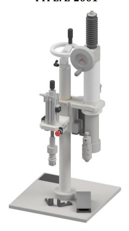
Z-2001 semi-automatic filling machine is a device used for filling aerosol containers with liquid (active substance). The amount of the dosed product is adjusted in the range of 5 - 510 ml (for product cylinder  $\emptyset$ 50 mm) with tolerance up to  $\pm$  0.5 ml<sup>1</sup>. The machine may be placed in the processing line for filling aerosol cans as a semiautomatic on-table model with manual control by an operator or as a self-acting unit in an Automatic Rotation Module.
