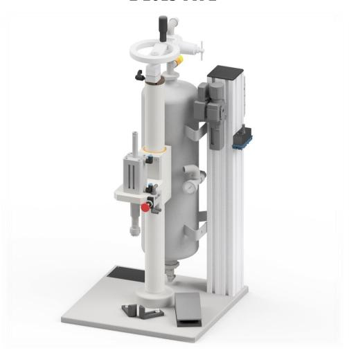
Semi-automatic  $CO_2/N_2$  Filling Machine Z-2013 is a device for filling aerosol containers with  $N_2/CO_2$  in gaseous form through a crimped valve. Device is powered and controlled by compressed air only and is equipped with gas accumulative tank. Filling pressure is limited to 1.6 MPa (16 bar). Machine can operate with Aerosol Valves or Bag-On-Valves, both in 1" standard.
