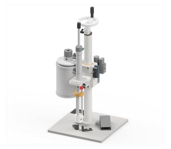
Semi-automatic Cleaning Machine Z-2059 is a device used for removing impurities from glass bottles before filling using blowing nozzle (cleaning head) combined with vacuum system. The bottles are to be provided manually. Device is powered and controlled by compressed air only. Device is equipped with its own vacuum generator and a separate filter, where all impurities and particles are stored.
