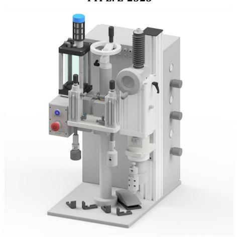
Z-2323 Semi-automatic BOV Filling Machine is a device designed for filling aerosol containers with liquid product through Bag-On-Valves crimped on the aerosol container. The amount of the dosed product is regulated in the range of  $5-510\,\mathrm{ml}$  (for product cylinder ø50 mm) with tolerance up to  $\pm$  0.5 ml1. Machine is equipped with 2 working heads:
