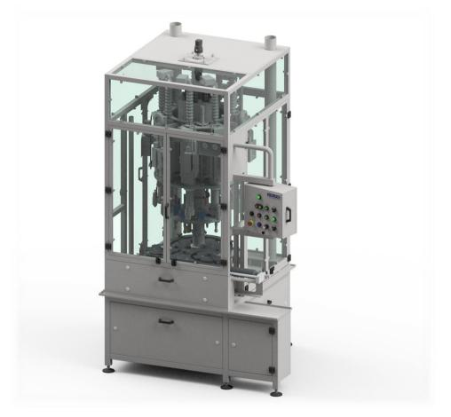
Rotational Gasifying Module ZIGMAT 180-1 is part of a production line and is intended for filling aerosol containers with a propellant through a crimped aerosol valve. The task is performed using 9 gasifying modules. The rated efficiency of the device is up to 180 pcs / minute. All working cycles take place during continuous (non-stop) rotary motion forced by the electric drive system.
