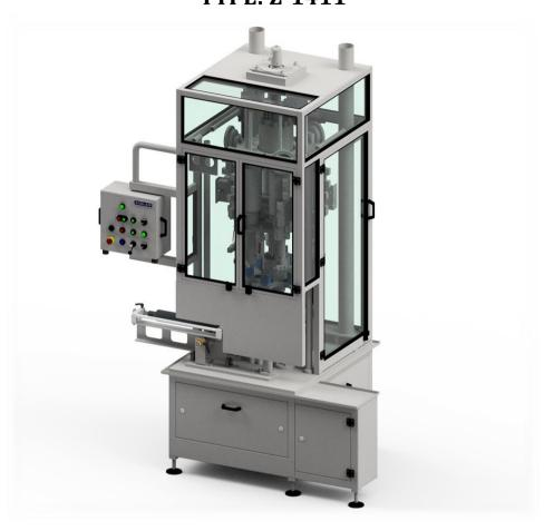
Rotational Gasifying Module ZIGMAT 120-1 Z-1411 type is part of a production line and is intended for filling aerosol containers with a propellant through a crimped aerosol valve. The task is performed using 6 gasifying modules. The rated efficiency of the device is up to 120 pcs / minute. All working cycles take place during continuous (non-stop) rotary motion forced by the electric drive system.
