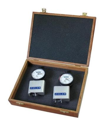
A set of instruments for crimping control. Each set consists of two measuring gauges and a ring for calibration:
