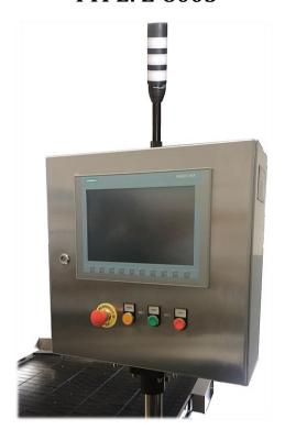
For the convenience of production line operators, Z-8003 Main Control Panel was installed at the Feeding Table Z-5200. This way, the operator responsible for the replenishment of empty containers has easy access to all necessary controls and buttons to control the operation of the equipment. He also has access to the HMI panel, which displays information about the current state of the production line.
