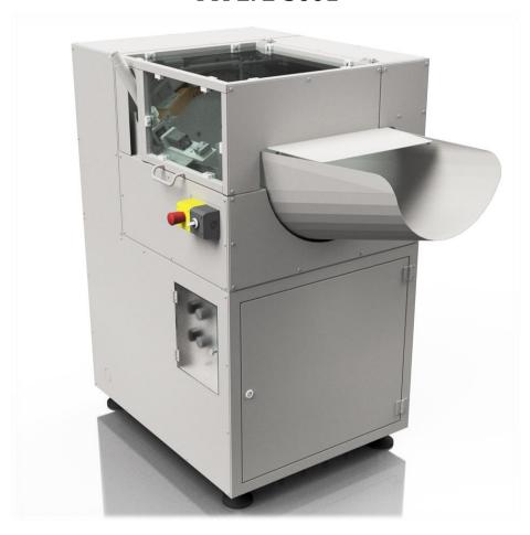
Valves sorter is a machine intended for feeding appropriately oriented (sorted) aerosol valves. Sorter is equipped with an electric drive of the sorting disc and the machine operation is controlled by a sensor system located at the sorting hopper and feeding guide. A special machine design allows for an optimal arrangement of sorted valves so that they enter the guide in right direction and may be immediately inserted onto the aerosol can.
