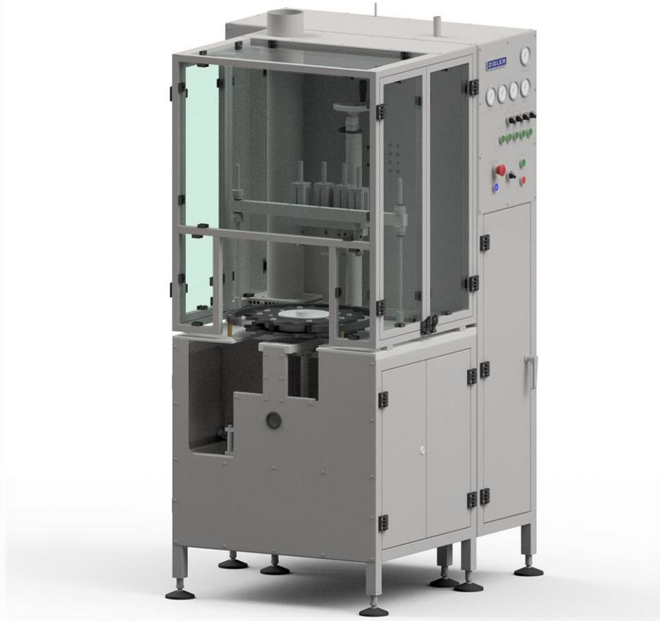
Gasifying Automatic Indexing Module Z-1033 is a machine which is a part of aerosol production line and is designed for perform following operations:
