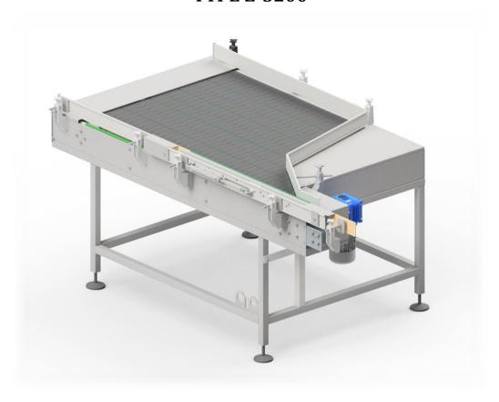
The Z-5200 type feeding table is an entry machine of automatic aerosol production line. The basic task of the feeding table is to provide continuous supply of empty containers in accordance to the demand of the production line. The table has been equipped with anti-jam rail preventing the containers from getting stuck at the narrowed output segment of the table.
