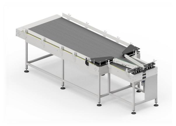
Feeding table Z-5215 is an input machine of the production line for the aerosol products manufacture. Basic function of the feeding table is to continuously supply empty cans as required by the production line. The table has been equipped with antijam rail preventing the containers from getting stuck at the narrowed output segment of the table.
