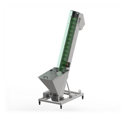
Z-4012 type Elevator is a machine intended for an automatic replenishment of sorting machine's hopper with small-sized semi-finished products (such as sprayheads). Elevator's large capacity hopper may by filled in cycles at long time intervals and does not require permanent operator's attention. The two machines interoperate by means of a common electronic control system.
