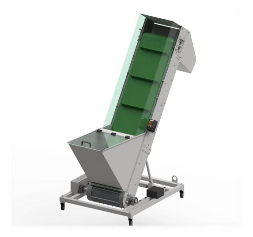
Z-4009 type Elevator is a machine intended for automatic replenishment of sorted small sized semi-finished products (such as aerosol valves, aerosol caps etc.) in sorting machine hopper. Elevator's large capacity hopper may by filled in cycles at long time intervals and does not require permanent operator's attention. Both machines interoperate by means of a common electronic control system.
