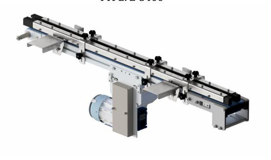
Main purpose of Conveyor Z-5400 is to transport small size elements like sprayheads, caps, screw caps, adapters etc. between the sorter and inserting/placing machine.
