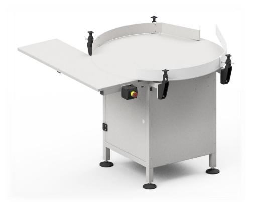
The Z-5102 Collecting Table is usually the last machine of the aerosol production lineup and is intended for receiving, bundling and packing finished products. It is equipped with a rotating worktop that allows the finished products to move towards the axis of the table, and an auxiliary table that allows for convenient placement of collective packages in order to fill them with manufactured articles.
