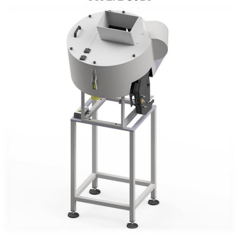
Caps sorter Z-3014 is a machine for automatic feeding properly oriented aerosol caps to cap conveyor, and further to the Cap Inserter Z-1491 unit. Device is equipped with a feeding hopper rotational whose task is cap reorientation. Automatic operation is controlled by a sorting hopper fill level sensor. The device is powered and controlled electrically. With removable sorting discs and adjustable guiding rails it is possible to work with different diameters of aerosol caps.
