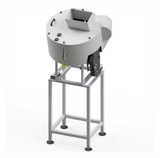
Caps Sorter Z-3004 is a device intended for feeding properly oriented (sorted) caps or screw caps to the conveyor cooperating with it. The device has been equipped with electric drive system and its operation is controlled by a system of sensors installed on sorting hopper and the conveyor. Special design of the device allows to optimally determine the orientation of sorted caps, thanks to which they enter the conveyor in a position allowing for their immediate placement onto the bottle or can.
