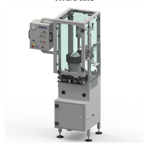
Caps Inserter Z-1102 is a machine designed to carry out one of the final phase of the aerosol production process - an insertion of Cap on the aerosol valve. Caps Inserter Z-1102 is designed for use with a conveyor, thanks to specially designed geometry of indexing wheel which collects the containers straight out from the belt.
