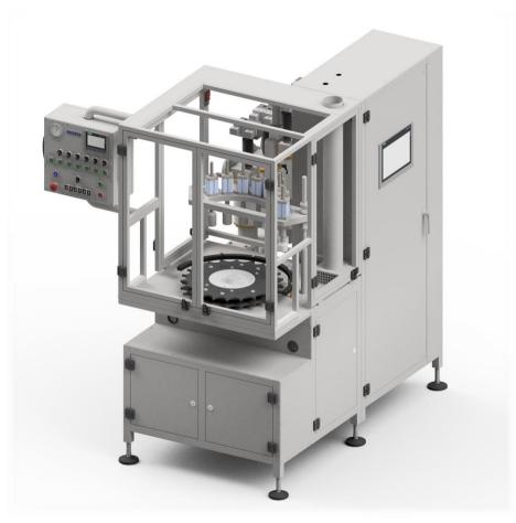
BOV Filling Automatic Indexing Module Z-1062 is a second machine of Automatic BOV Aerosol Production Line and is intended to perform following operations:
