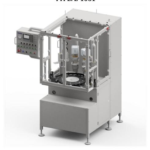
BOV Closing and Testing Automatic Indexing Module Z-1061 is a first machine of Automatic BOV Aerosol Production Line and is intended to perform following operations:
