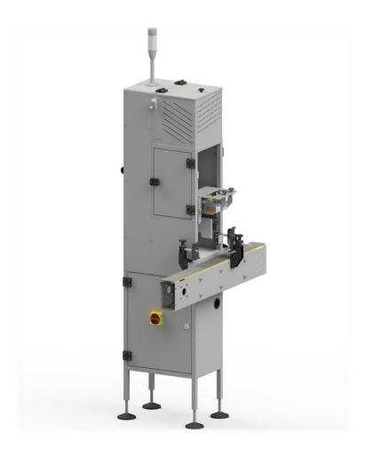
Balls Feeding Automatic Module Z-1553 is intended for inserting steel balls (or glass ones as an option) into aerosol cans. The device has the option to feed one or two balls in one working cycle. Device is powered pneumatically and electrically and is designed to work with the conveyor. In standard, the device is adapted to support one diameter of balls.
